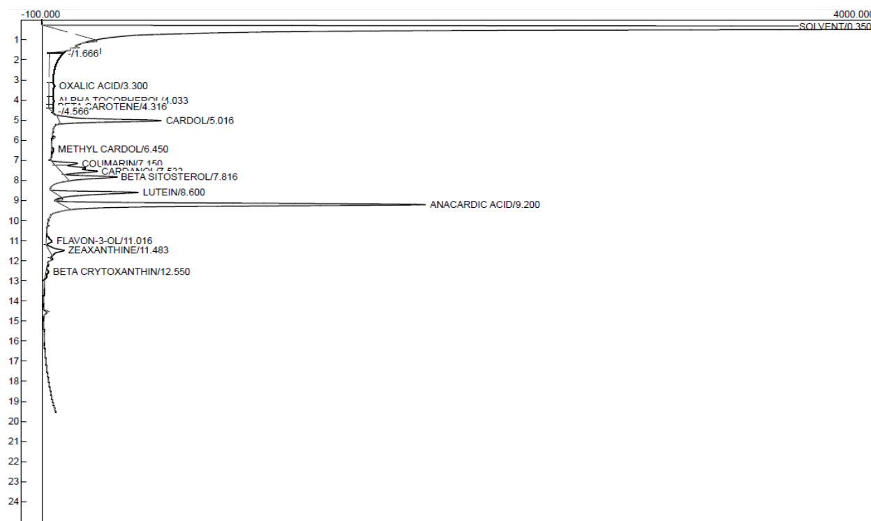
Fig.5 Gas Chromatography-Flame ionization detector (GC-FID) chromatogram of Anacardium occidentale nut shell extract
